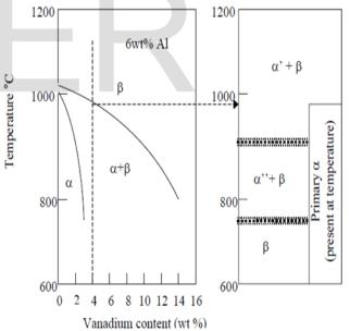
Fig No.2 A schematic illustration of microstructures occurring in Ti-6A1-4V after quenching from different temperatures [5]
