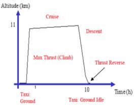
Fig 3 Typical Flight Cycle [2]
