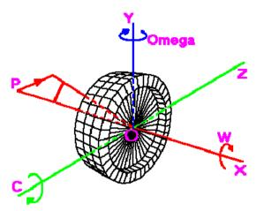
Fig.4 Forces created by the spinning moments of engines during takeoff [2]
